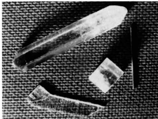
Fig. 1. \text{Li}_{1-x}\text{H}_x\text{IO}_3 single crystals (scale 3:1).
